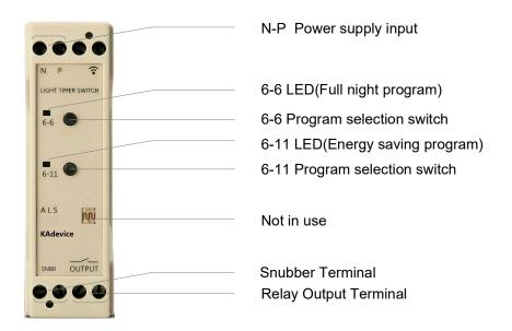
**N-P Power supply Input:** Input supply voltage ranges from 24v to 264v AC or DC. Recommended to use a circuit breaker 2-pole between the input power source and the timer for safety. LED flicker every 10sec once indicating timer power ON.
