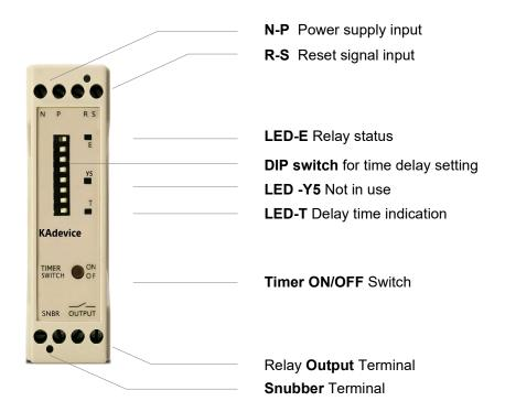
**N-P Power supply Input:** Input supply voltage ranges from 24v to 230v AC or DC. Recommended to use a circuit breaker 2-pole between the input power source and controller for safety. LED T flicker every 5sec once indicating timer power ON.
