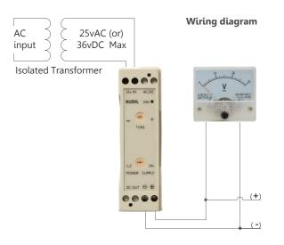
Din rail mountable switching power supply, It is designed for low voltage application. Adjustable output voltage and capable of drive a 2 Amps load with excellent line and load regulation. The model DAV is competitively price and it can operate continuously at its maximum rated output and is overload protected. This manual provides the information to help the maximum performance and longest life for this power supply.
